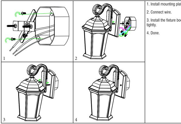
3. Install the fixture body and screw nut
