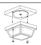
\*Push the shade straight into ceiling pan, and then twist the two mounting screws tightly.
