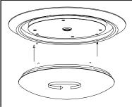
\*Push the shade straight into ceiling pan, and then twist the shade into place
